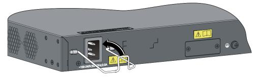
Figure 3-18 Connect an AC power cord to a vertical AC power socket (2)
